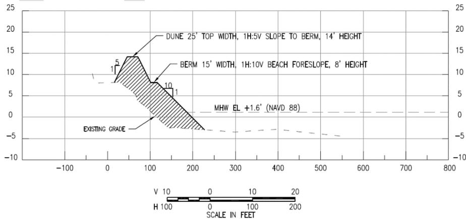
Figure 24 - Dredged Material Placement Locations Design Template (Lewes)
