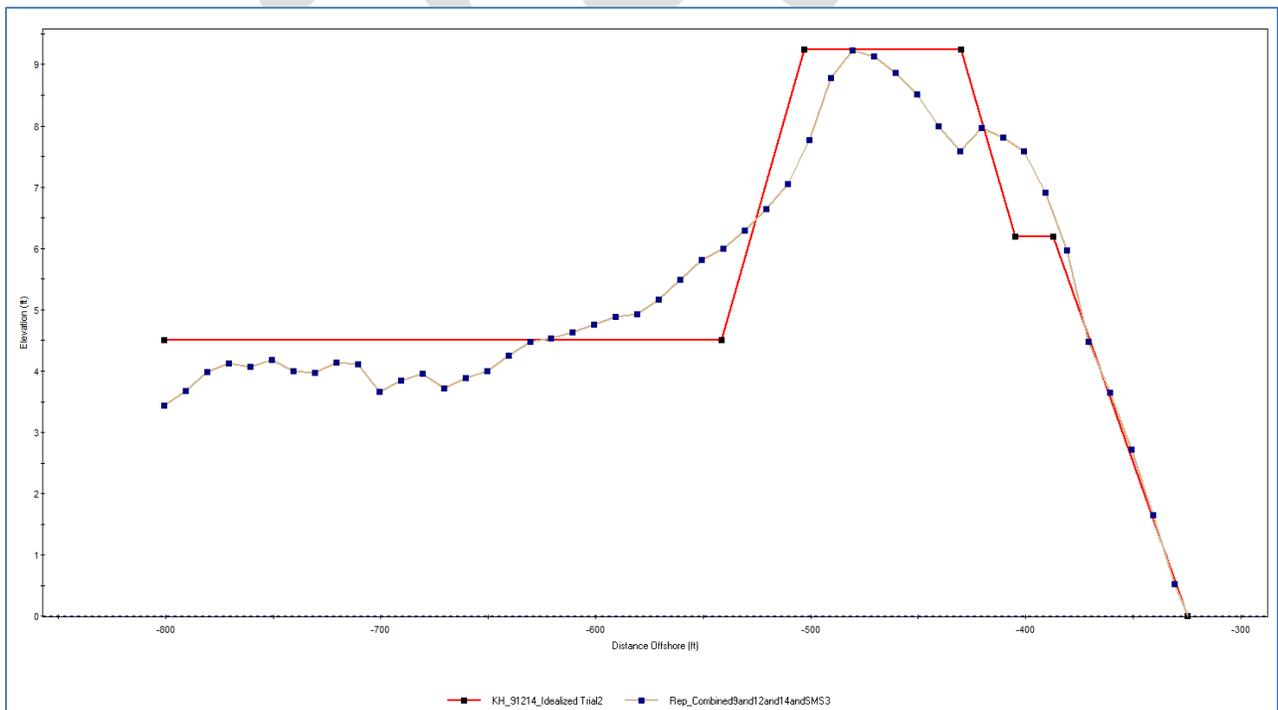
Figure 12 – Enlarged view of Representative and idealized profile for Kitts Hummock (#2)
