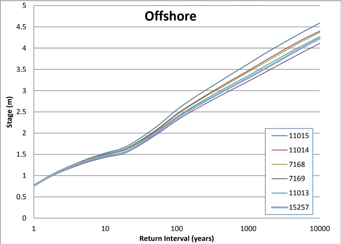
Figure 26 - Stage frequency curves at NACCS stations in Delaware Bay near DMU sites
