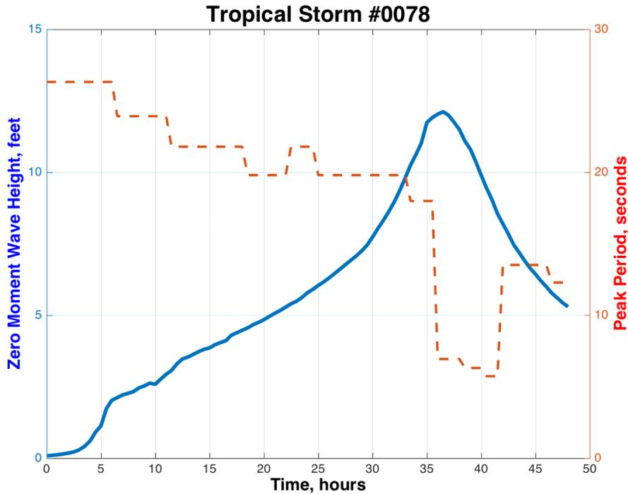
Figure 33 - Wave height and period time series for a selected 200-yr event (Storm 78).
