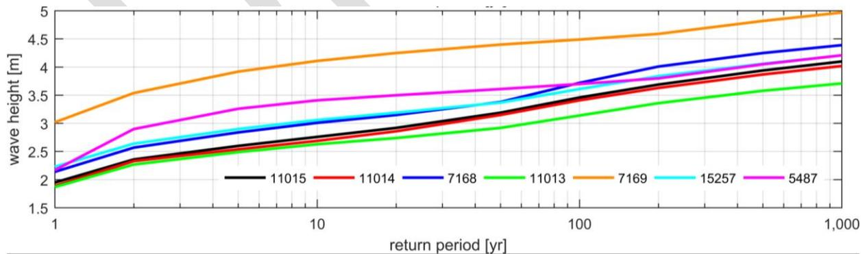
Figure 27 – Comparison of wave height at NACCS stations in Delaware Bay near DMU sites
