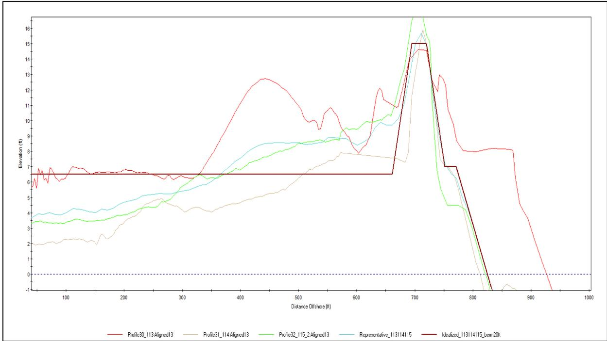
Figure 18 - Zoom view of Profiles 30-32, the representative profile, and the idealized profile
